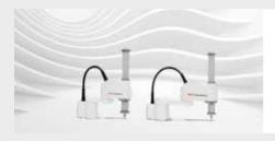
Featuring a white epoxy coating, IP54, NSF-H1 food-grade grease and anti-rust bolts, the SR-3iA/C and the SR-6iA/C are the ideal choice for tray food and cleanroom applications.
